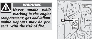
1. Engine oil - 2. Battery 3. Brake fluid - 4. Windscreen washer fluid - 5. Engine coolant -**6.** Power steering fluid
