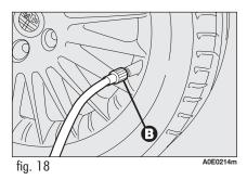
loosen tyre inflation valve cap, take out the filler hose A-fig. 17 and screw the ring nut B-fig. 18 on the tyre valve;
