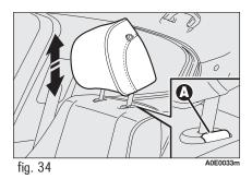
WARNING Remember that the head restraints should be adjusted to support the back of your head and not your neck. Only in this position do they exert their protective action. To optimise head restraint protective action, adjust the seat back upright and keep your head as close as possible to the head restraint.
