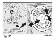
WARNING Any adjustment of the steering wheel position must be carried out only with the car stationary and the engine turned off.
