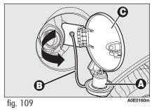
When refuelling, position the cap on the device inside the flap as shown in the figure.
