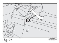
To extend it, take it out of the reel by taking tongue **A-fig. 21** and secure ends **B-fig. 22** into the two housings **C-fig. 23** (one per side) located on the roof of the car.
