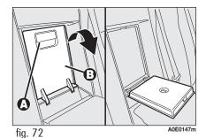
To open the lid B, switch A-fig. 73 (accessible from the boot) shall be set
