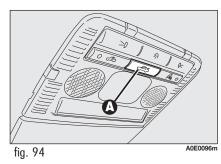
On certain versions, improper boot closing is indicated by the instrument panel warning light  $\ominus$ , whereas on other versions the symbol  $\overleftrightarrow$  and a message are displayed (see section "Warning lights and messages").
