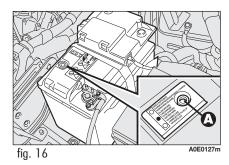
Should the battery be not fitted with battery charge inspection device (optical electrolyte indicator), inspection operations shall be carried out by skilled personnel only.
