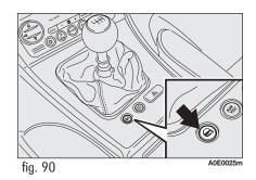
With key removed the led will turn off after about 2 minutes.
