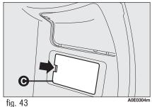
open the fuse box lid C-fig. 43 working in the point shown by the arrow.
