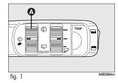
The rear window wiper stops working a few strokes after releasing the ring nut; a further stroke after about 6 seconds completes the wiping operation.
