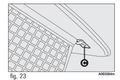
To roll up the net, release ends **B-fig. 22** from housings **C-fig. 23** and guide it during rolling.
