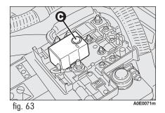
The switch is located inside the fuse box at battery positive terminal.
