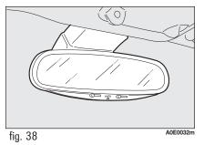
Certain versions are fitted with electrochromic mirror **fig. 38**. The electrochromic function is turned on/off by pressing button **ON/OFF** in the lower section of the mirror. When engaging reverse, the mirror will always set to daylight colouring.
