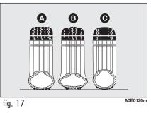
Incorrect pressure causes abnormal tyre wear **fig. 17**:
