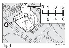
**IMPORTANT** The car can only be put into reverse gear when it has stopped moving completely. With the engine running, before engaging the reverse, wait at least 3 seconds with the clutch pedal fully down to prevent damage and grating of the gears.
