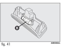
replace the bulb **B-fig. 41** releasing it from the side contacts making sure that the new bulb is correctly clamped between the contacts;
