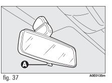
Using lever **A-fig. 37** the mirror can be adjusted to two different positions: normal or antiglare.
