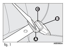
To unfasten the seat belts, press button **C**. Guide the seat belt with your hand while it is rewinding, to prevent it from twisting.
