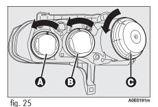
WARNING After replacement, refit the covers correctly checking that they are properly secured.
