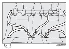
When the car is parked on a steep slope the reel mechanism may block; this is normal. The reel mechanism prevents the webbing coming out when it is jerked or if the car brakes sharply, in a collision or when cornering at high speed.
