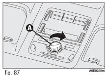
**IMPORTANT** Top comfort position with sunroof open is obtained by turning selector **A-fig. 87** to position.
