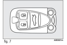
Button a shall be used for central opening of doors and fuel cap with alarm deactivation (where provided).
