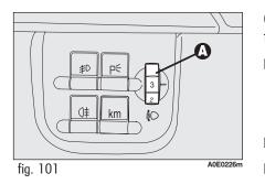
In this event, to adjust the headlight slant use control **A-fig. 101** set on the button control panel near the steering wheel.
