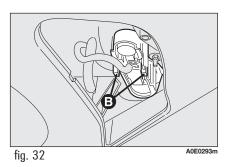
remove the bulb holder unit by pressing the retaining tabs **B-fig. 32**;
