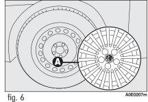
Remove the wheel cap A-fig. 6 (only versions with steel rims);
