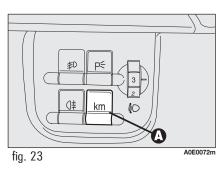
To reset the trip meter (or mi), press for long button **A-fig. 23** during displaying.
