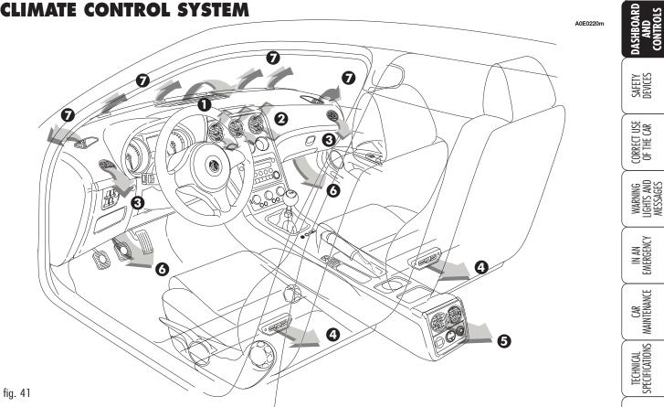
Upper vent - 2 Adjustable and swivel central vents - 3 Adjustable and swivel side vents - 4 Lower vents for rear seats 5 Adjustable and swivel air vents for rear seats (where provided) - 6 Lower vents for front seats - 7 Windscreen and front windows demisting/defrosting vents.
