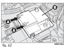
Resetting the power supply cut-off switch (where provided)
