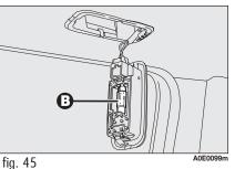
replace the bulb **B-fig. 45** releasing it from the side contacts making sure that the new bulb is correctly clamped between the contacts.
