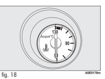
**IMPORTANT** The pointer can reach the red area also for a sum of unfavourable conditions, i.e.: slow speed, uphill, fully laden or towing a trailer with hot outside temperature.
