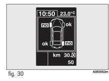
On versions fitted with T.P.M.S. system (Tyre pressure Monitoring System) (see paragraph "T.P.M.S. system" in this section), after Trip A and Trip B info, the screen with tyre pressure condition is displayed (see **fig. 30**).
