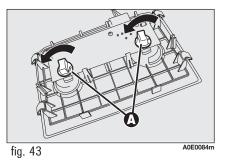
turn the 2 bulb holders A-fig. 43 counter-clockwise, remove and replace bulbs.
