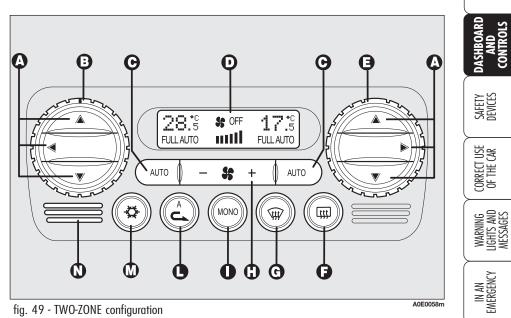
I - Button for activating the MONO function (alignment of set temperatures), corresponding to driver's one;
