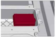
The number identifying the electrical component corresponding to each fuse is shown on the cover
