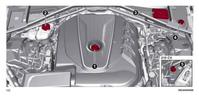
1. Engine oil filler 2. Engine coolant reservoir cap 3. Brake fluid reservoir cap access cover 4. Windscreen/headlights washer fluid reservoir cap 5. Secondary engine cooling reservoir plug
