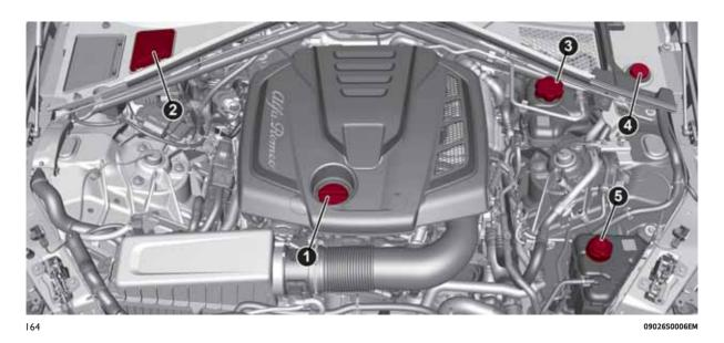
1. Engine oil filler 2. Brake fluid reservoir cap access cover 3. Primary engine cooling reservoir plug 4. Windscreen/headlights washer fluid reservoir cap 5. Secondary engine cooling reservoir plug
