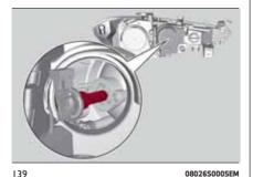
remove the bulb by sliding it off the bulb holder;
