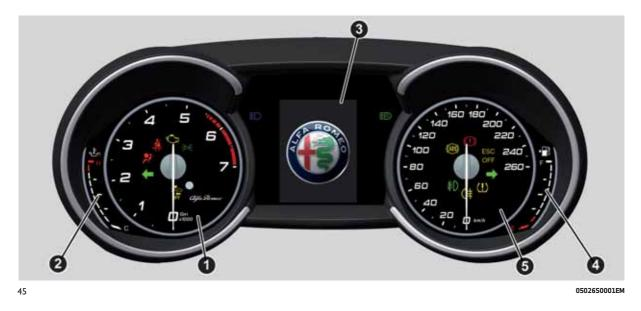
1. Rev counter 2. Digital engine oil temperature gauge with overheating warning light 3. TFT Display 4. Digital fuel level gauge (the triangle on the left side of the symbol indicates the side of the vehicle with the fuel filler) 5. Speedometer (speed indicator)
