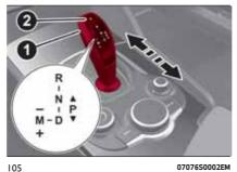
The positions diagram is illustrated on the top of the lever.
