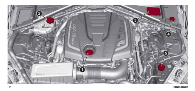
1. Engine oil filler 2. Primary engine cooling reservoir plug 3. Brake fluid reservoir cap access cover 4. Windscreen/headlights washer fluid reservoir cap 5. Secondary engine cooling reservoir plug
