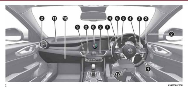
1. Light switch; 2. Air diffusers; 3. Left stalk; 4. Steering wheel controls; 5. Instrument panel; 6. Steering wheel; 7. Right stalk; 8. Connect; 9. Automatic dual-zone climate control system; 10. Glove compartment; 11. Passenger side air bag; 12. Bonnet release lever.
