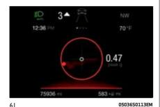
The displayed parameters are related to vehicle stability, the graphs illustrate the trend of the longitudinal/lateral accelerations (G-meter information), considering gravitational acceleration as a reference unit
