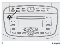
The doors will be locked only if all the doors are properly shut. In the absence of electrical power supply (e.g. blown fuse, battery disconnected, etc.) it is still possible to lock the doors manually. IMPORTANT With central locking on, pulling the internal handle of one of the doors will unlock that door. When 20 km/h are exceeded, all the doors will be automatically locked (if the dedicated display Setup Menu function has been activated).
