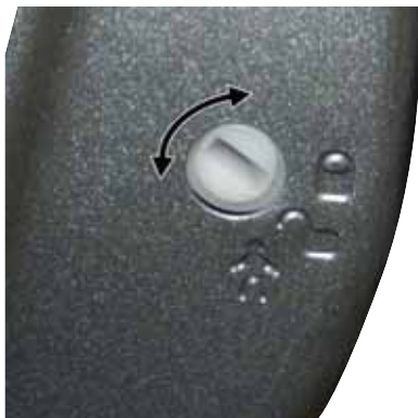
Child-Protection Door Lock Function
