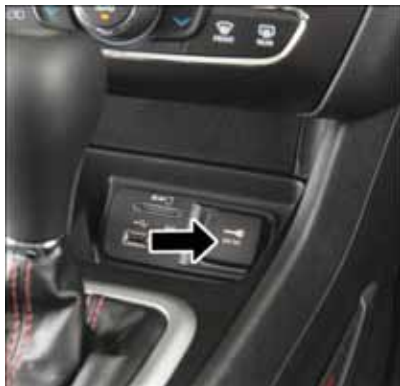
Front Power Outlet
