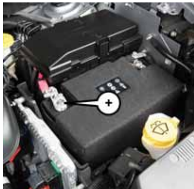
Positive Battery Post
