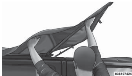
4. Engage the header latches.
