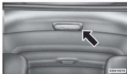
Flashlight Location/Press To Release
