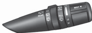
Wiper/Washer Control Lever
