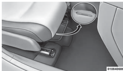
Right Front Body VIN Location
