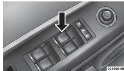
Power Window Switch Location
