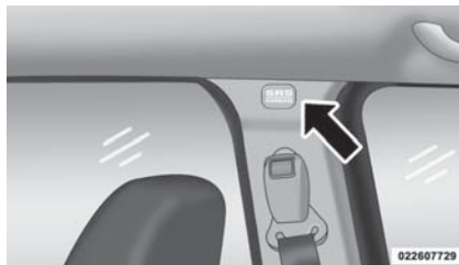
Side Curtain Air Bag Label Location
