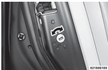
Child-Protection Door Lock Function
