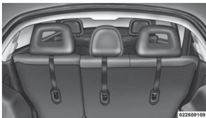
Rear Seat Tether Anchors
