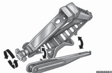
Removing Jack Handle From Jack
