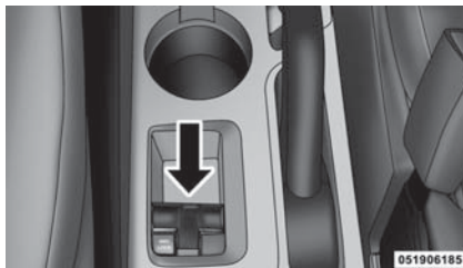
Four-Wheel Drive Switch
