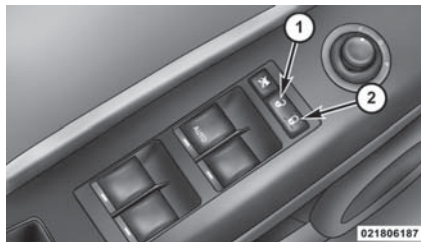
Driver Power Door Lock Switch
