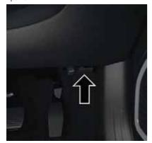
**Hood Release Location (Underneath** Instrument Panel)
