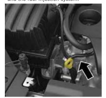
Suitable Engine Ground (Example Engine Shown)
