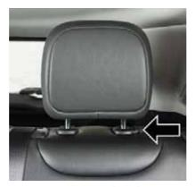
Outboard Head Restraint Adjustment Button
