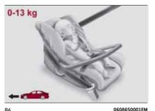
The child restraint system is secured by the vehicle seat belts, as shown in fig. 86 and it must restrain the child in turn with its own belts.
