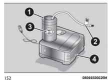
compressor 4 complete with pressure gauge and connectors;
