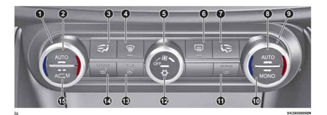
side air distribution selection button; 4. MAX-DEF function activation button (rapid defrosting/demisting); 5. Fan speed adjustment knob; 6. Heated rear window on/off button; 7. Passenger side air distribution selection button; 8. Passenger side AUTO function activation button (automatic operation); 9. Passenger side temperature adjustment knob; 10. MONO function button (set temperature alignment) driver/passenger side; 11. Passenger side seat heater activation button; (where provided, see
