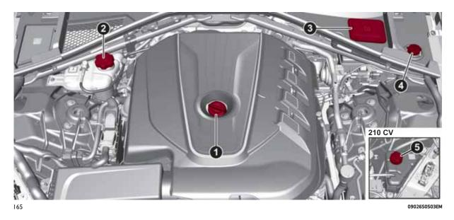
1. Engine oil filler 2. Primary engine cooling reservoir plug 3. Brake fluid reservoir plug access cover 4. Windscreen/headlights washer fluid reservoir plug 5. Secondary engine cooling reservoir plug
