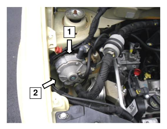
Get a small mirror to identify the code printed on the pressure regulator (1)
